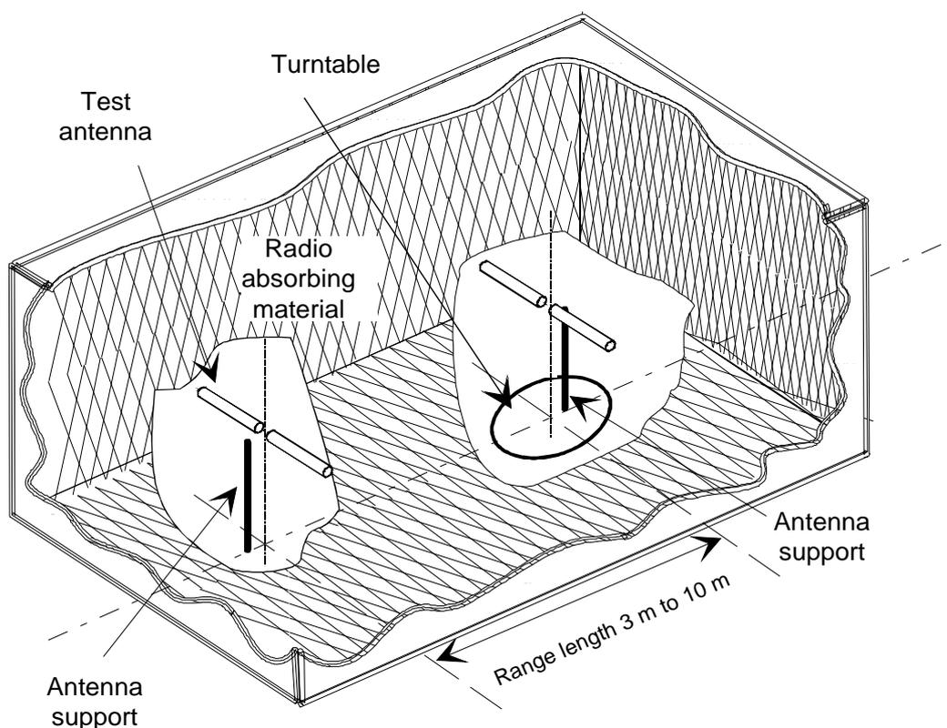
Figure D.1: A typical anechoic chamber
